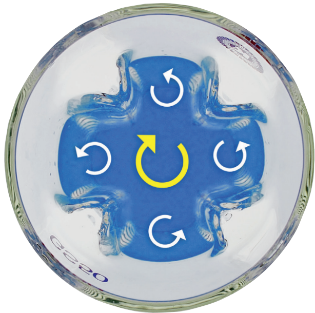
GS vessel principle (viewed from top)
